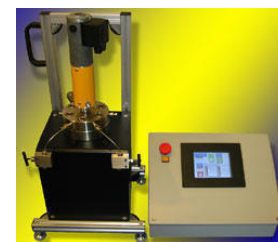
HPR Series Reactor with RxTrol™ Controller ▲
